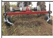
**BEDSHAPER** Build raised beds up to 6" high and 32" wide with this tool. Also useful for some hilling applications. Available with Disk Hillers (pictured) or Furrow Plows, both POTATO DIGGER PLOW: fully adjustable. Has drag chain to level off bed top. Min. 20" tall
