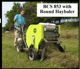
Walk-Behind Tractors are extremely popular in many parts of the world where farm sizes are small due to population density, rugged terrain, and land use patterns. The concept is simple: just like a conventional 4-wheel tractor, the walk-behind allows the ability to use ONE MACHINE to perform a variety of agricultural, lawn, garden, landscaping, municipal and commercial jobs by utilizing many different
