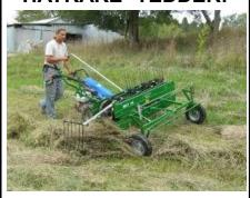
PTO-driven, this side delivery rake is fully agricultural quality & can even be used for de-thatching & light scarification when lowered completely. Rakes have a steering system built-in, for effortless handling. Converts to a Tedder in 30 seconds with a simple frame adjustment. 40 & 60" Sizes. 8hp &
