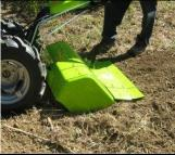
TILLER DEPTH SYSTEM: This full-width "roller" attaches to the back of the 30" tiller implements, PRECISELY controlling depth and producing perfect pre-tamped, level seed-
